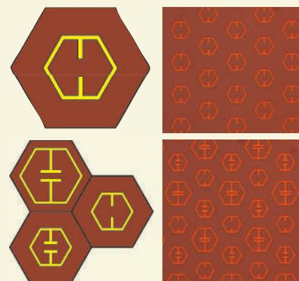
resonances of their metamaterials were a good match for those of vitamin H. This match could therefore form the basis of a biodetector. Bingham *et al.* have found that their multi-subunit tiling techniques can create multi-resonator metamaterials that can be used as biodetectors. But that is not all. Their metamaterials could potentially detect hazardous chemicals.
